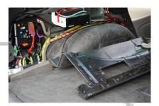
Now carefully remove the foam which is settled around the DVD-RTI Unit, and fold it out. You will need to remove a black clasp, by turning it 1 bit clockwise.
