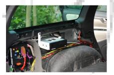
Now, remove the Torx bolts (4 pieces) from the DVD-RTi Unit, which makes it possible to remove the unit from its holder. Please carefully pull the unit forward. Do not create to much tension on the cables! Then remove the Canbus/Power cable (looks the same as in the CFE-RTI Connection set) from the DVD-Unit.
