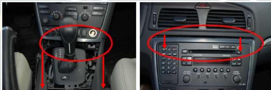
Now turn/move the radio on top or in front (towards you) of the gear shifter so you can reach the back of the radio. Put towels (plenty!) on top of the gear shifter and panels to avoid damages!
