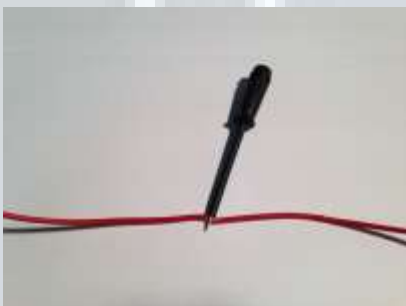
Insert a pinny-sharp object and split the wires
