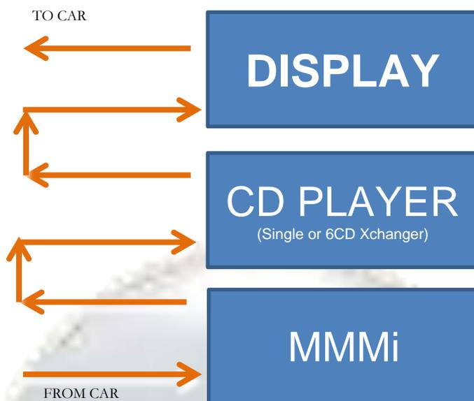
To create this connection, you need to disconnect the incoming MOST cable from the connector at the CD player.
